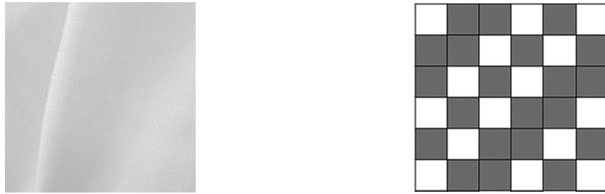
Figure 1: White bamboo fabric: surface of white bamboo fabric (left), performance of rapport 2/1 twill weave of white bamboo fabric (right)
