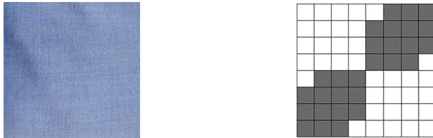
Figure 2: Blue bamboo fabric: surface of blue bamboo fabric (left), performance of rapport of white bamboo fabric (right)
