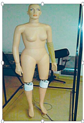
Figure 2: Thermal manikin Maria with left forearm covered with sample of firefighter protective clothing
